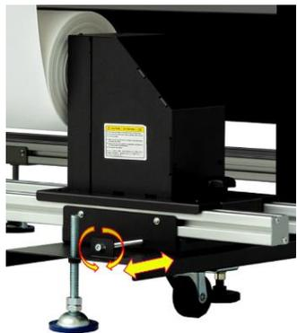
Position adjustment mechanism for roll units
